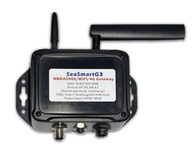
The multi-function weather-resist data port auto switches from Serial mode to USB mode when plugged into a compatible PC/Laptop and is electrically isolated from the NMEA 2000 bus. Serial mode allows legacy NMEA 0183 equipment an upgrade path to NMEA 2000 using the PushSmart<sup>™</sup> Protocol while USB mode provides an isolated protective interface to PCs running marine instrumentation and chart plotting applications such as the vDash real-time virtual dashboard.
