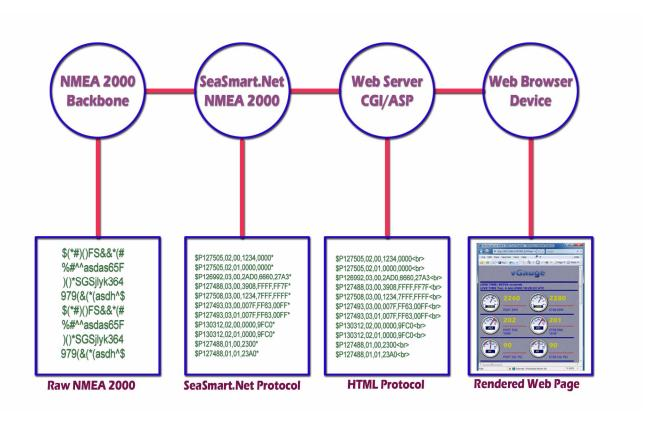
Raw NMEA 2000 data is read directly from the Backbone and translated to SeaSmart.Net protocol so it can be passed on and processed by Web Servers. The Web Servers then in turn format the data into HTML friendly documents which can be retrieved by common Browser based devices. The Browsers render the live data into graphical displays that are easily customizable via standard Web design tools.
