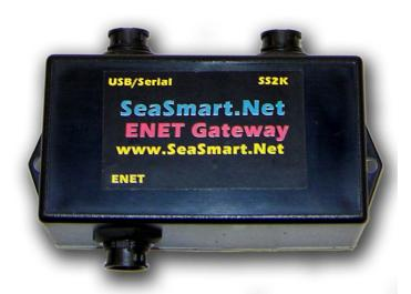
Multi-function weather-resist data ports feature secure twist-lock connections and sealed cables for reliable performance. Separate NMEA 2000 and RS232 ports allow legacy NMEA 0183/AIS devices to share a common Ethernet TCP/IP connection. Full protocol suite is provided for DHCP, Static IP, FTP, HTTP, UDP, TELNET and more. All network configurations are performed via embedded Web Pages from any browser enabled device.
